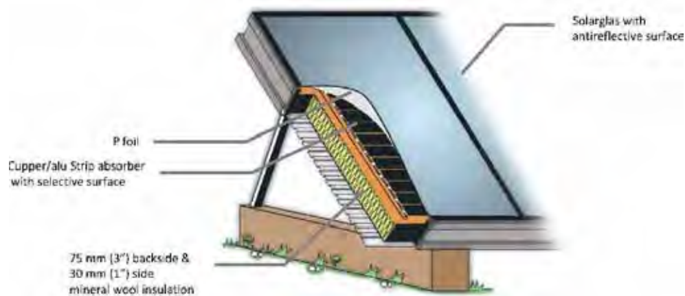
Figure A-24. Cross section of the ARCON HT collector.
