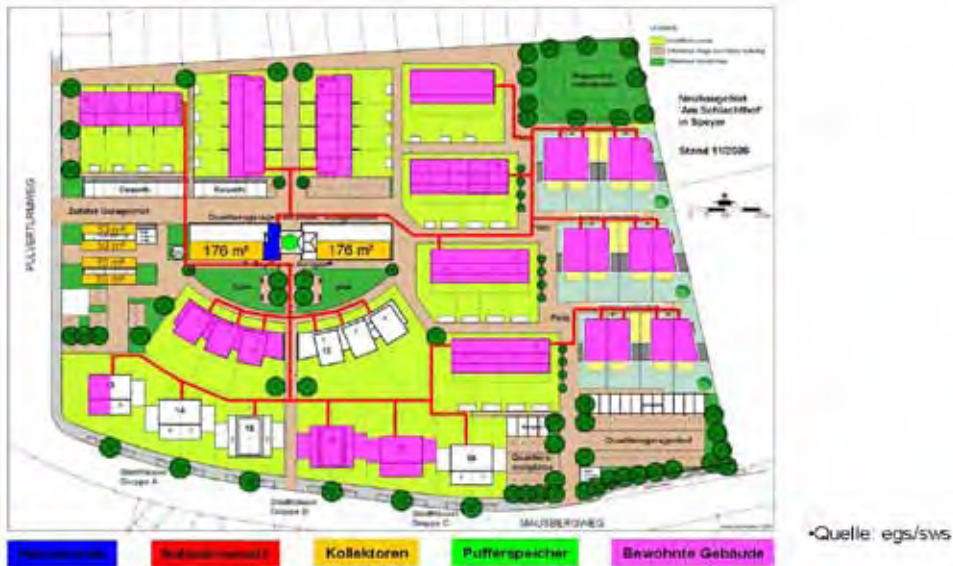
Figure A-42. District heating Speyer “Old Slaughterhouse.”
