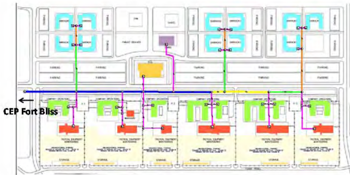
Figure B-4. Fort Bliss network model of the DH system.
