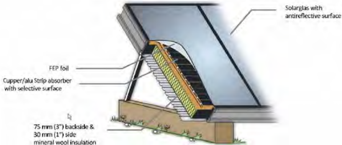
Figure A-21. Cross-section of the ARCON HT collector.
