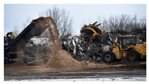
A front end loader grabs tree waste material and puts it into the hopper of a grinder at Environmental Wood Supply in St. Paul on Wednesday, Jan. 22, 2020. The tree waste generated in this region is processed into fuel for use at St. Paul Congeneration, which produces renewable electricity and heat. State leaders attended a briefing at the site Wednesday. (Jean Pieri / Pioneer Press)
